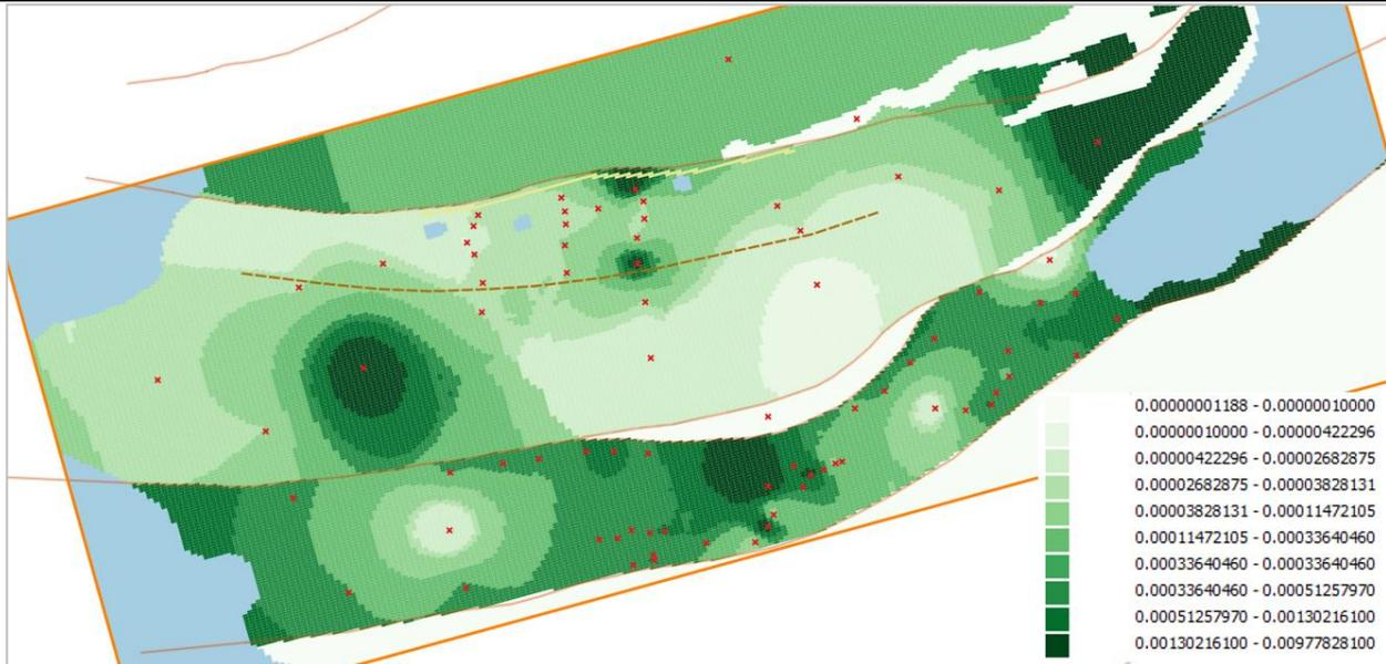
Figure 40. Hydraulic conductivity distribution obtained from the PP value adjustments (in m/s).
