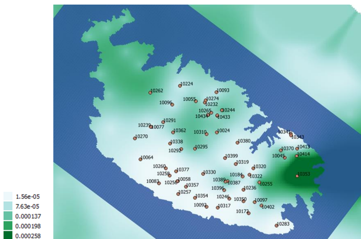
Figure 16. Reconstructed hydraulic conductivity distribution, given by the interpolation of available data plus fictitious points to cover the whole model domain.
