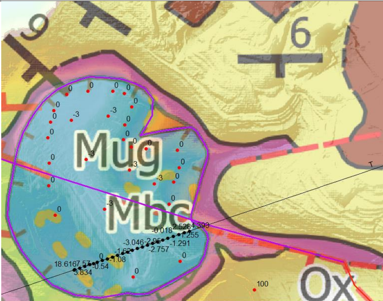
Figure 8. Example of sinkhole mapped boundary in north-western seaside of Gozo island, utilized as interpolation “barrier”, together with cross sections (black dots) and dummies points (red dots) constraining the interpolation of sinkhole bottom.
