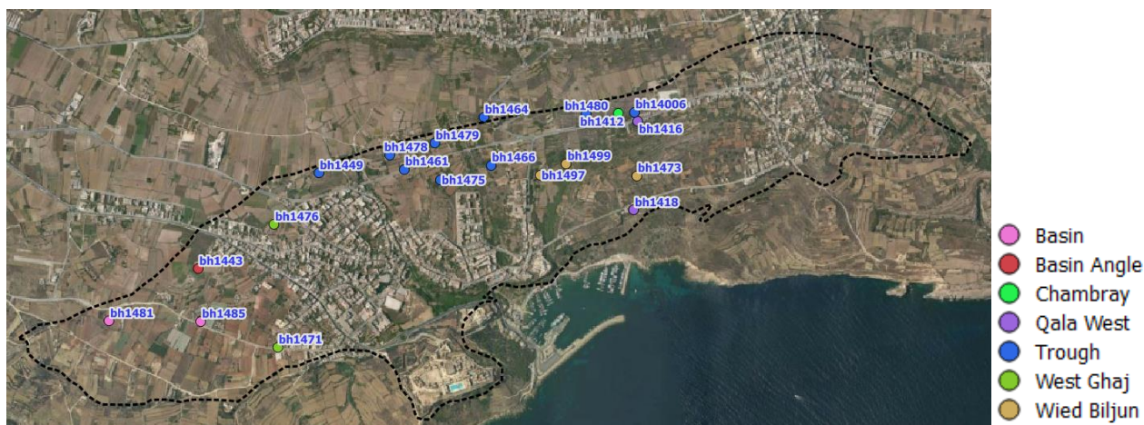
Figure 82. Position of the 18 target points used for sensitivity and calibration, colored according to the region classification identified in (Costain, 1958).
