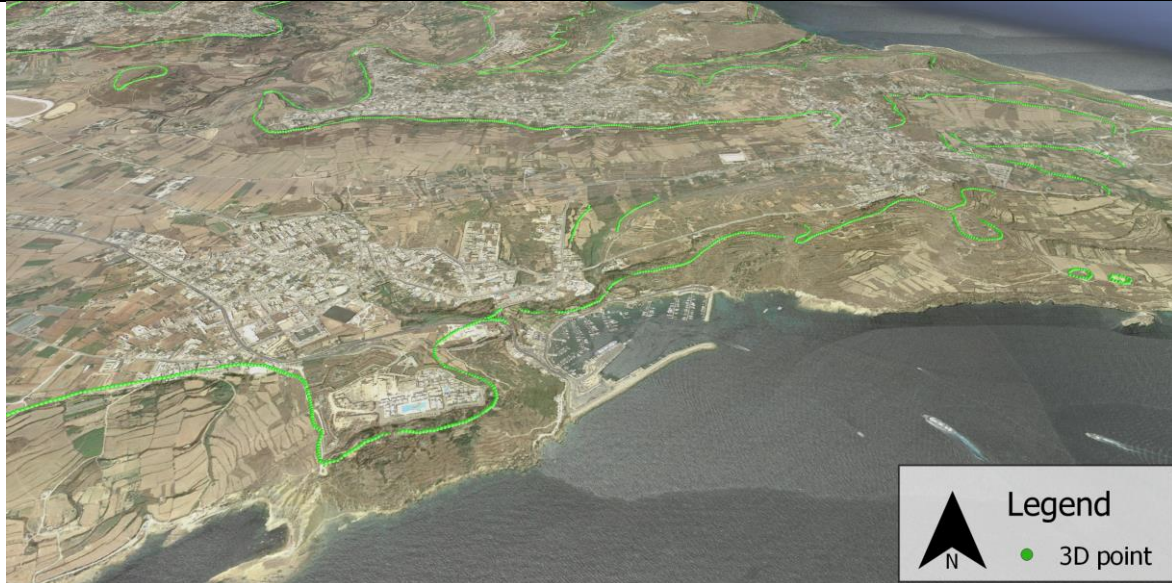
Figure 5. Example of 3D points extracted from geological boundaries used to interpolate the bottom boundary of the UCL formation (south east Gozo).
