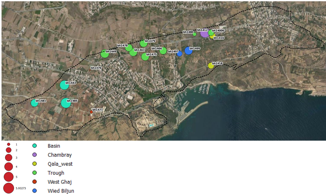
Figure 87. Bubble plots of absolute residuals (in m). Points are colored according to the different region classification, according to Costain (1958).
