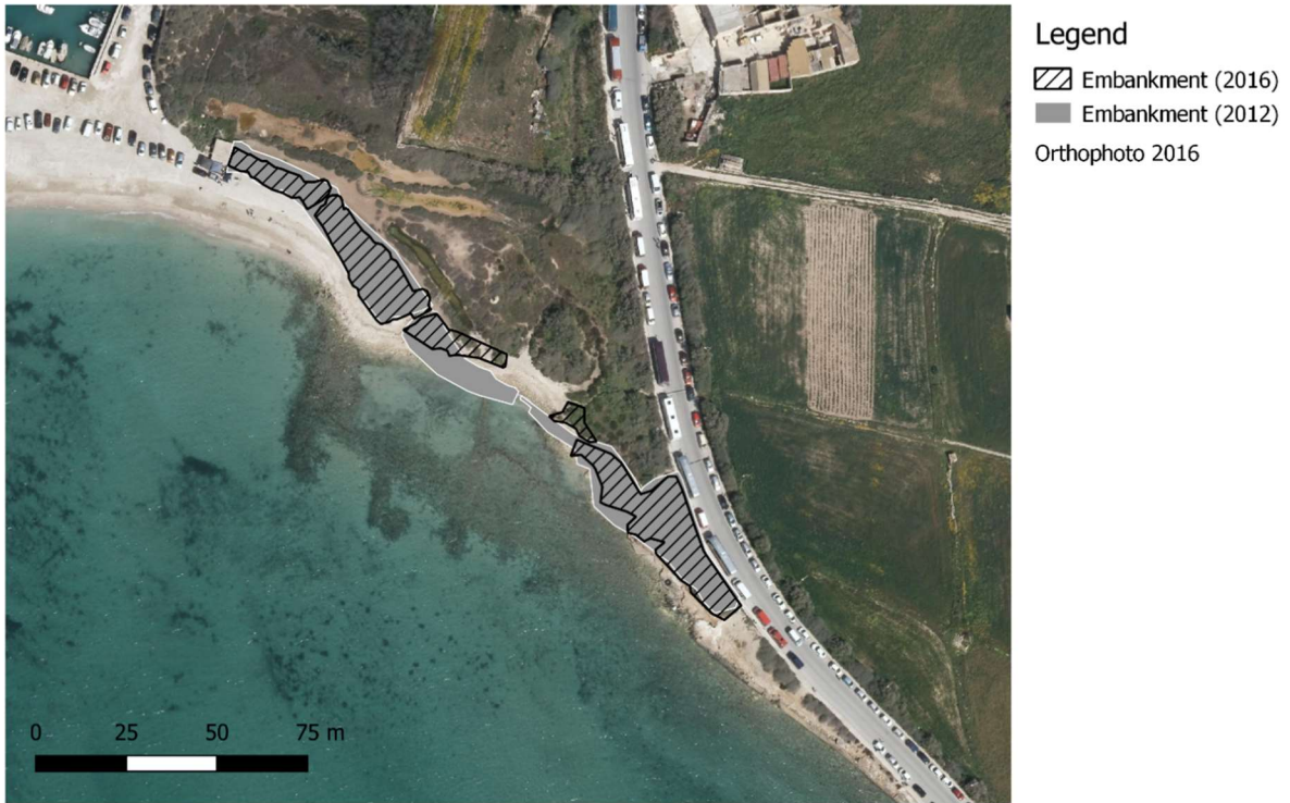
Figure 15 – Difference between the embankment extent based on orthophotos from the years 2012 and 2016 (Source: Planning Authority).
